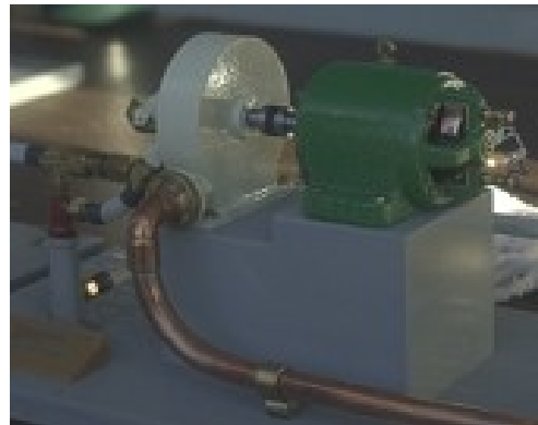
Left: Jerry Bartlow's engine with Hackworth gear.
